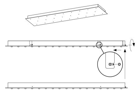
Screw in the locking screw completely.
